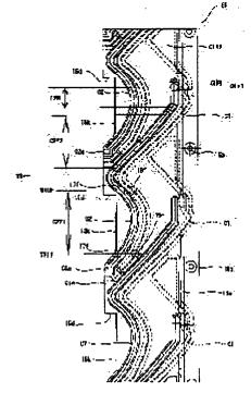
one of the front group lens or the rear group lens passes through the partial area of the cam groove for another lens group and faces the cam groove part for the one lens group.
